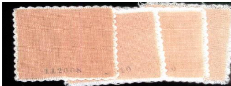
Figure 2: Example of a wash trail at 40°C, 8dH with EMPA 112 Detergent without Amylase (left) and Detergent plus increasing amount of Amylase (as of 2nd from the left to the right)
