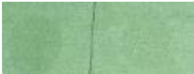
Figure 3: Example of a wash trail at 40°C, 8dH with an Olive Oil Stain. Detergent without a Lipase (left) and Detergent plus a Lipase (right)
